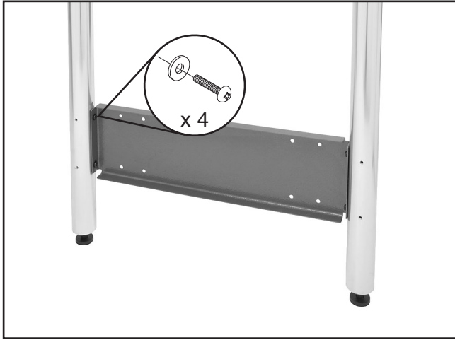
Figure 19. Installing shelf end plate on extension table legs.
